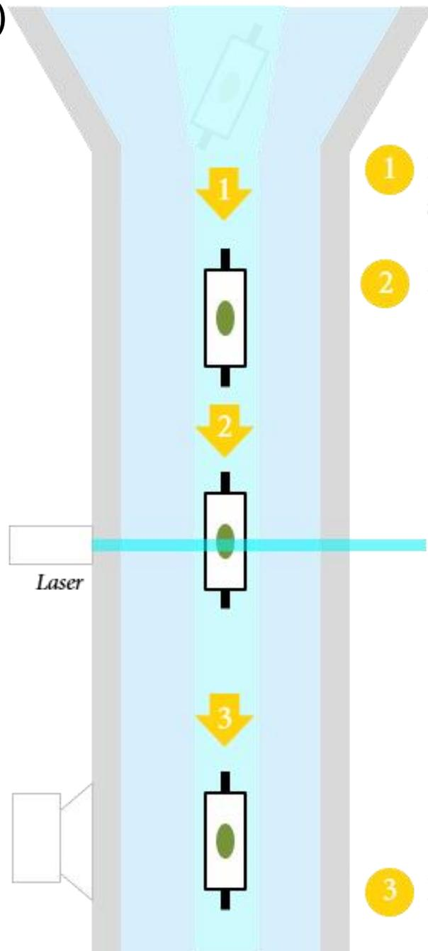
1 Hydronamic alignment of analyzed particles
