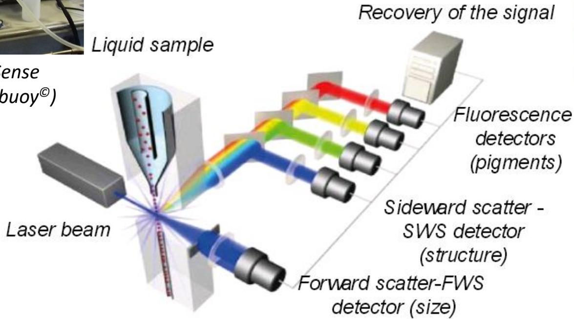
Principle of the PSFCM: from 1 to 800  $\mu\text{m}$  width... and few mm length
