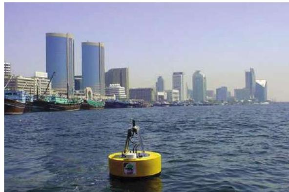
YSI Water Quality Monitoring buoy on Dubai Creek.
